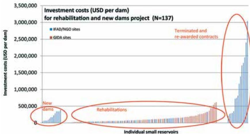
FIGURE 7. Investment costs for rehabilitation and new dam construction (USD).
