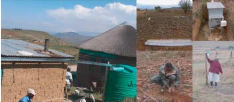
*Rooftop run-off harvesting, setting up run-off plots, TDR access tubes and rain gauges.*
