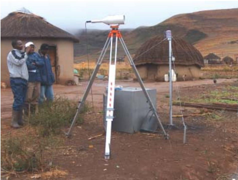
A Scintillometer measures sensible heat flux along a transect (typically less than 10km) from which the latent heat flux (total evaporation) can be computed as a residual in the surface energy balance equation after measuring the soil heat flux. The surface energy balance equation is given as:
