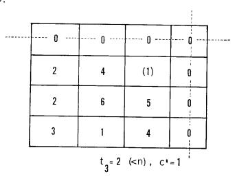
Third Step. The smallest element c' not included in the lines  $t_3$  is subtracted from every element in the matrix  $(c_{ij})$  but is then added back to those elements which lie along one of the lines. Note that for an element cij lying along one such line,
