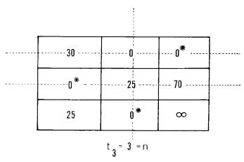
Optimal solution reached, as indicated by asterisks
