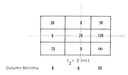
Step 2: Column minima subtracted from column elements
