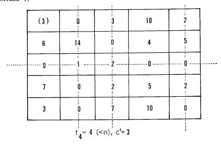
Step 4: Minimum element subtracted from all elements and added back to rows and columns covered by  $t_{\mathbf{4}}$
