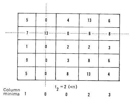
Step 2: Column minima subtracted from column elements
