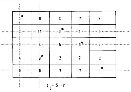
Optimal solution reached, as indicated by asterisks
