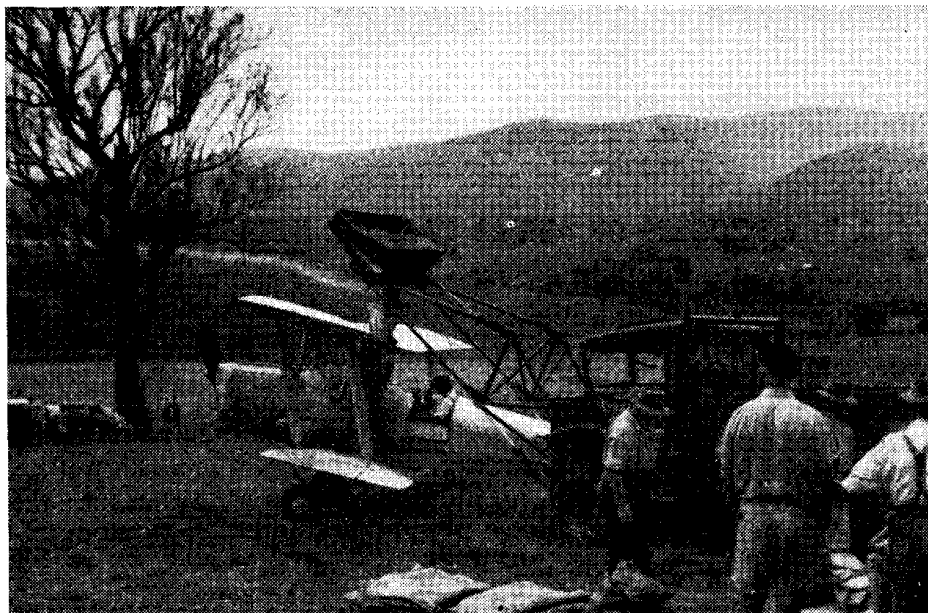
Loading of Tiger Moth DH 82 from ground dump of bagged superphosphate Each bag has to be emptied into the truck-mounted hopper. An improved technique is shown in the following photograph. Note trail of fertiliser from spreading aircraft behind the tree.
