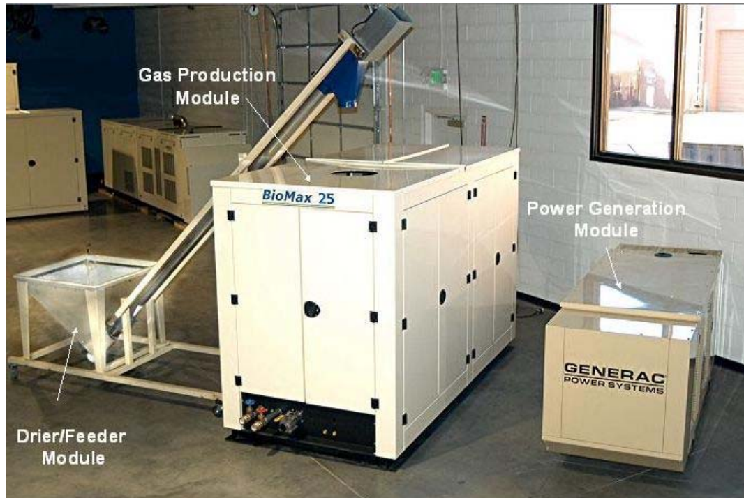
Figure - BioMax Modular Biopower System (25 kWe) manufactured by Community Power (CO)
