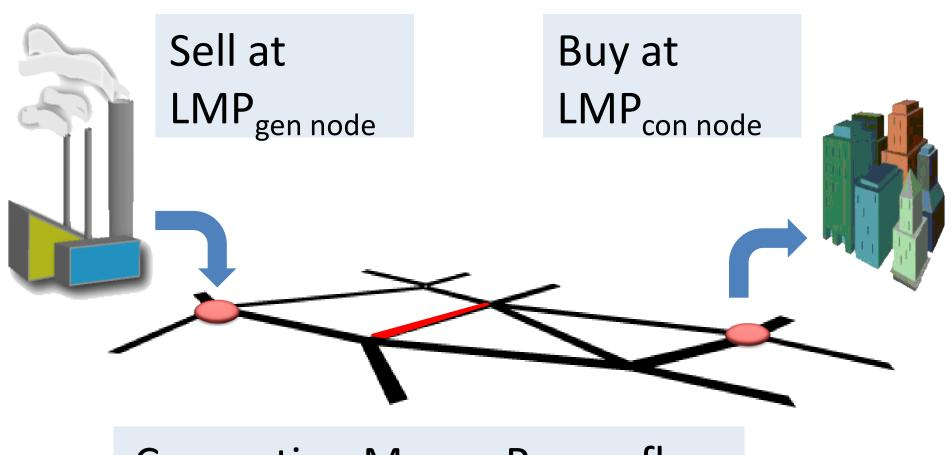
**Congestion Means Power flow** on the line at its rated capacity
