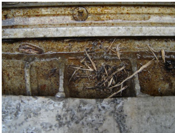
Figure 4: Moisture, rust and pallet splinters on a container floor
