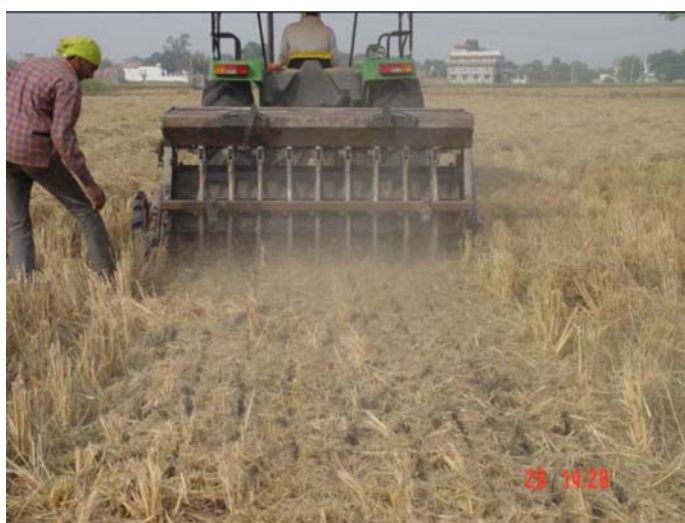
Figure 5. Turbo Happy Seeder (photo Dasmesh Mechanical Works)
