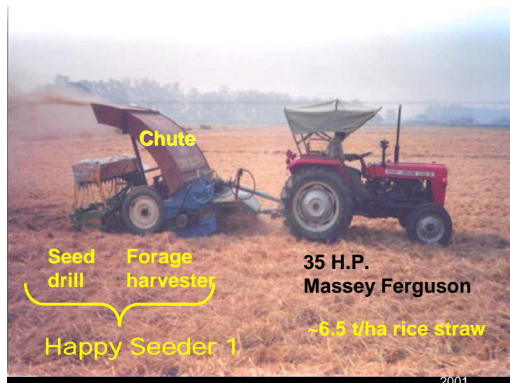
Figure 3. The Original Happy Seeder (photo J. Blackwell)
