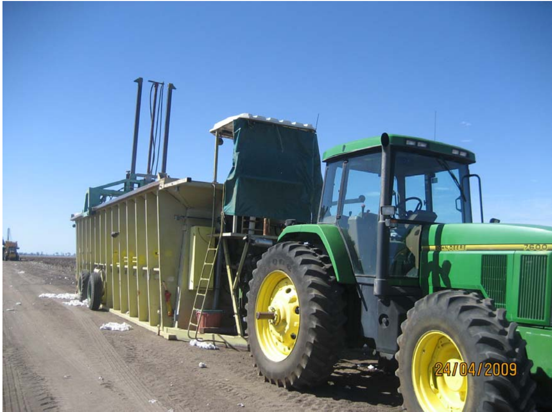
Figure 6: Transport of cotton to the gin in Australia is completely mechanized. This shows cotton being compacted on a farm for transport to the gin.
