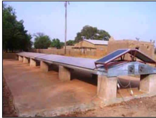
Figure 5 IER Solar powered shea nut dryer, Lafiala, Mali (Perakis, Fieldwork, 2007)
