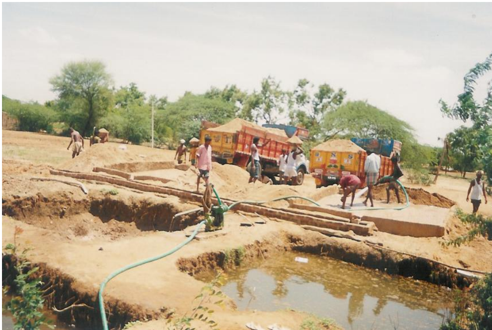
Sand being washed using compressor pump to remove red sting as white color sand fetches high price, Gauribidanur taluk, Karnataka, 2003
