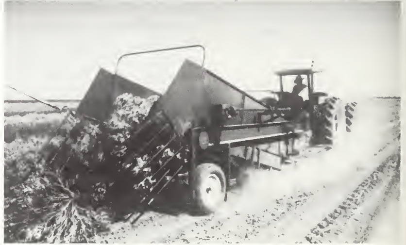
Figure 8. Implement designed to undercut and then lift guayule shrub onto the soil surface.
