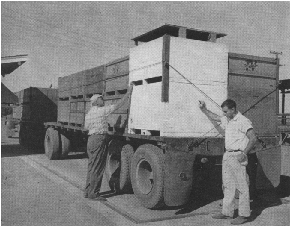
Fig. 1. White bulk bins contain instruments for measuring vibration characteristics of different types of trucks.
