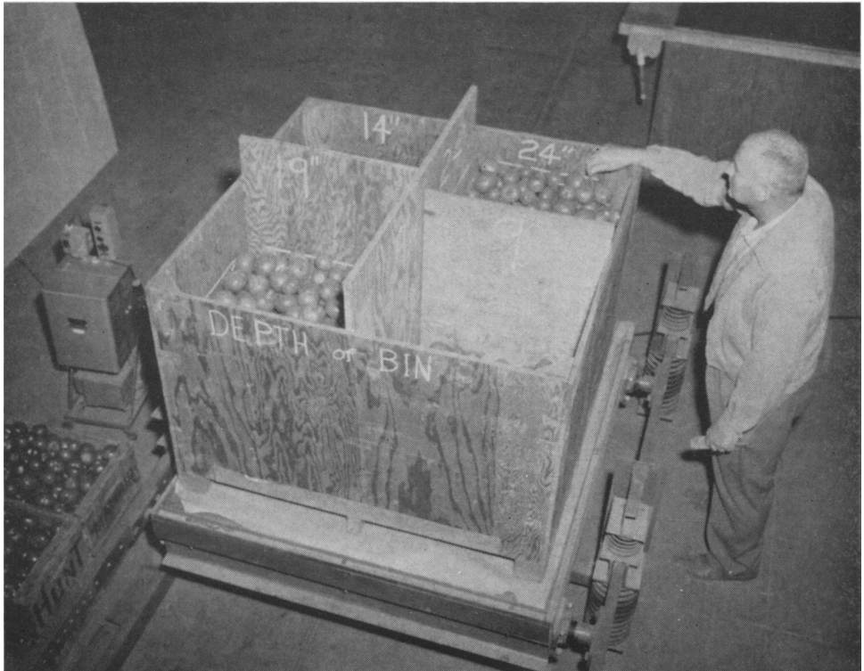
Fig. 3. U.C. 145 tomatoes on simulated-transport vibrator in the laboratory.
