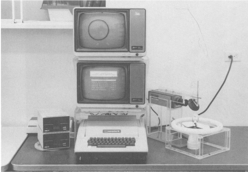
Fig. 1. This computerized tracking system includes an Apple II Plus microcomputer, a video camera, two monitors, two disk drives, and a Silentyper printer to establish the activity levels of strains of M. occidentalis .
