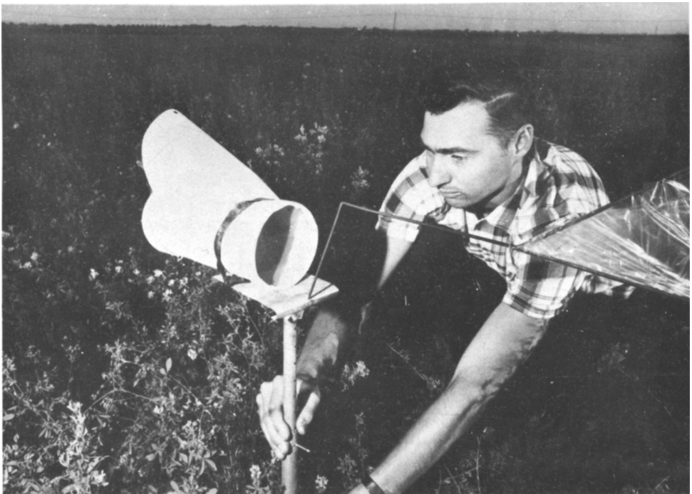
Fig. 12. Omni trap used to capture male Lygus hesperus . The trap was mounted on a platform capable of weathervaning. The airscoop (see text) was positioned on top of the trap as shown.
