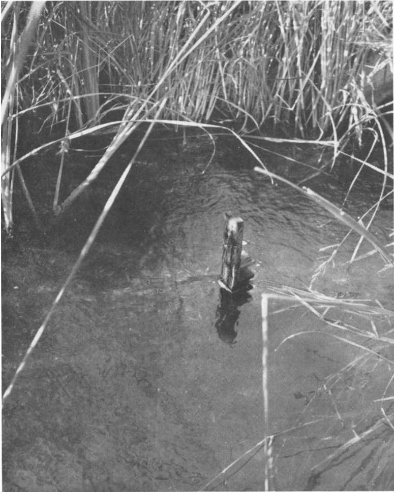
Fig. 211. Varied-level stake located in moving water below a weir box in a second-year rice field (Field H).
