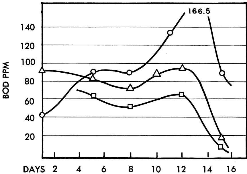
Fig. 16. Biochemical oxygen demand data obtained in laboratory from effluents of continuous growth units.
