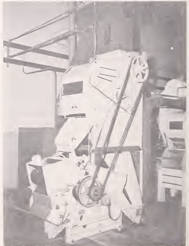
FIGURE 3.—Small-scale gin stand (20-saw).
