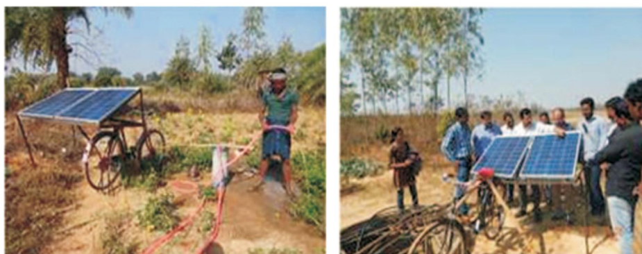
Fig. 3. Solar Energy operated DC Pump for irrigation adopted by Harsha trust
