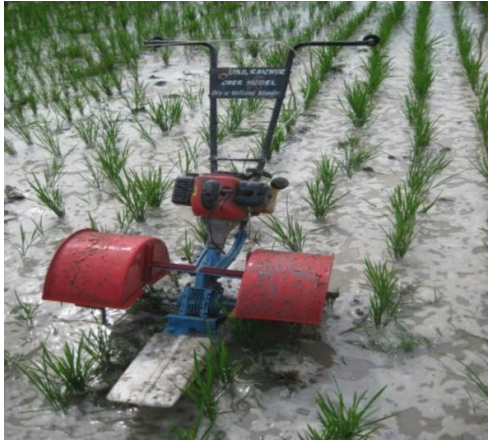
Fig. 1. Wet land power weeder
