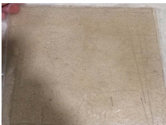
Figure 4. Biocomposite made of cellulose microfibers from sugarcane straw and polylactic acid.
