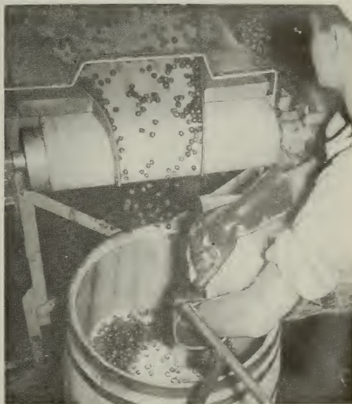
Figure 8. - Sugar is added to the fruit in the barrel while it is continually rocked or shaken to get an even distribution throughout.
