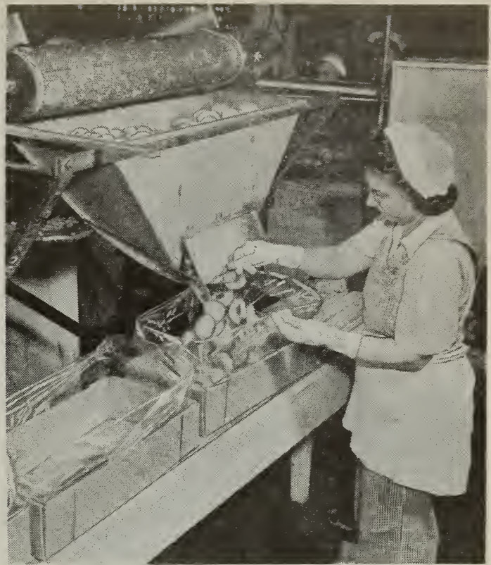
Figure 2. - Peaches are treated in sirup, then released from the hopper into cellophane-lined cartons which protect them from loss of moisture, freshness, and flavor.
