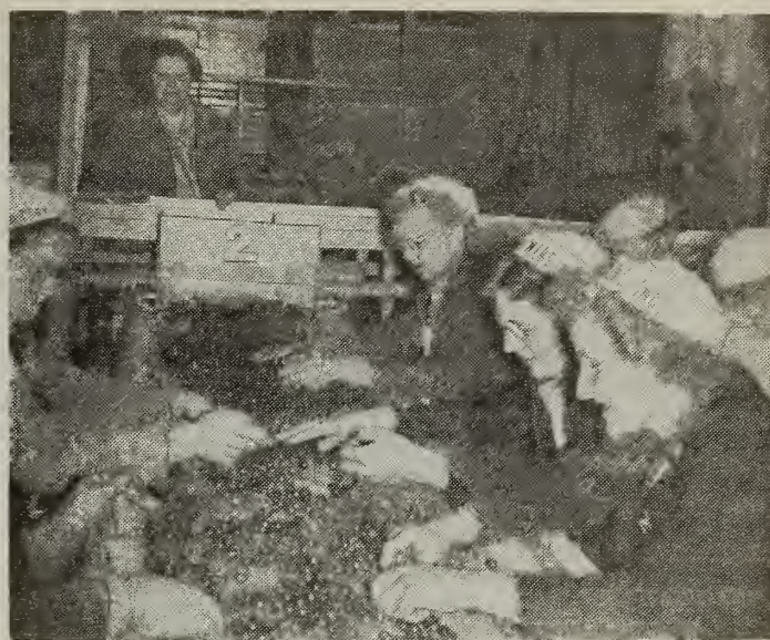
Figure 6. - Culls and undesirable pieces must be removed by hand.
