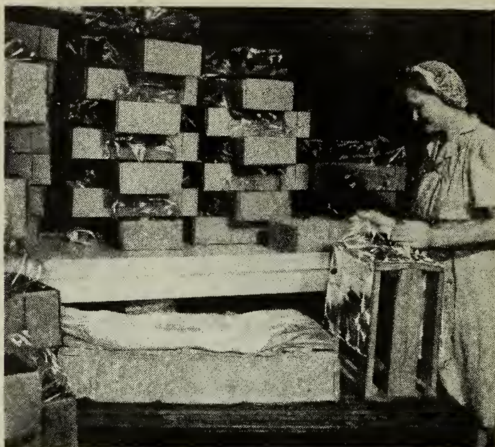
Figure 9. - The cellophane pouch is shaped over this specially designed mandrel, which may be collapsed for storage when not in use, and the carton is then fitted over the liner.
