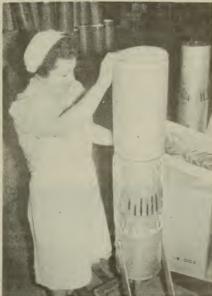
Figure 10. - This cylindrical container, used extensively as a wartime substitute for tin, is also fitted with a cellophane liner.
