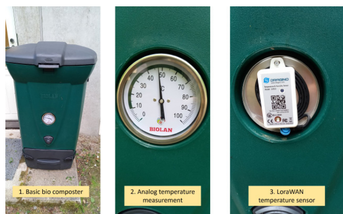
Figure 2: 1. Basic bio composter; 2. Analogue temperature measurement; 3. LoRaWAN temperature sensor.
