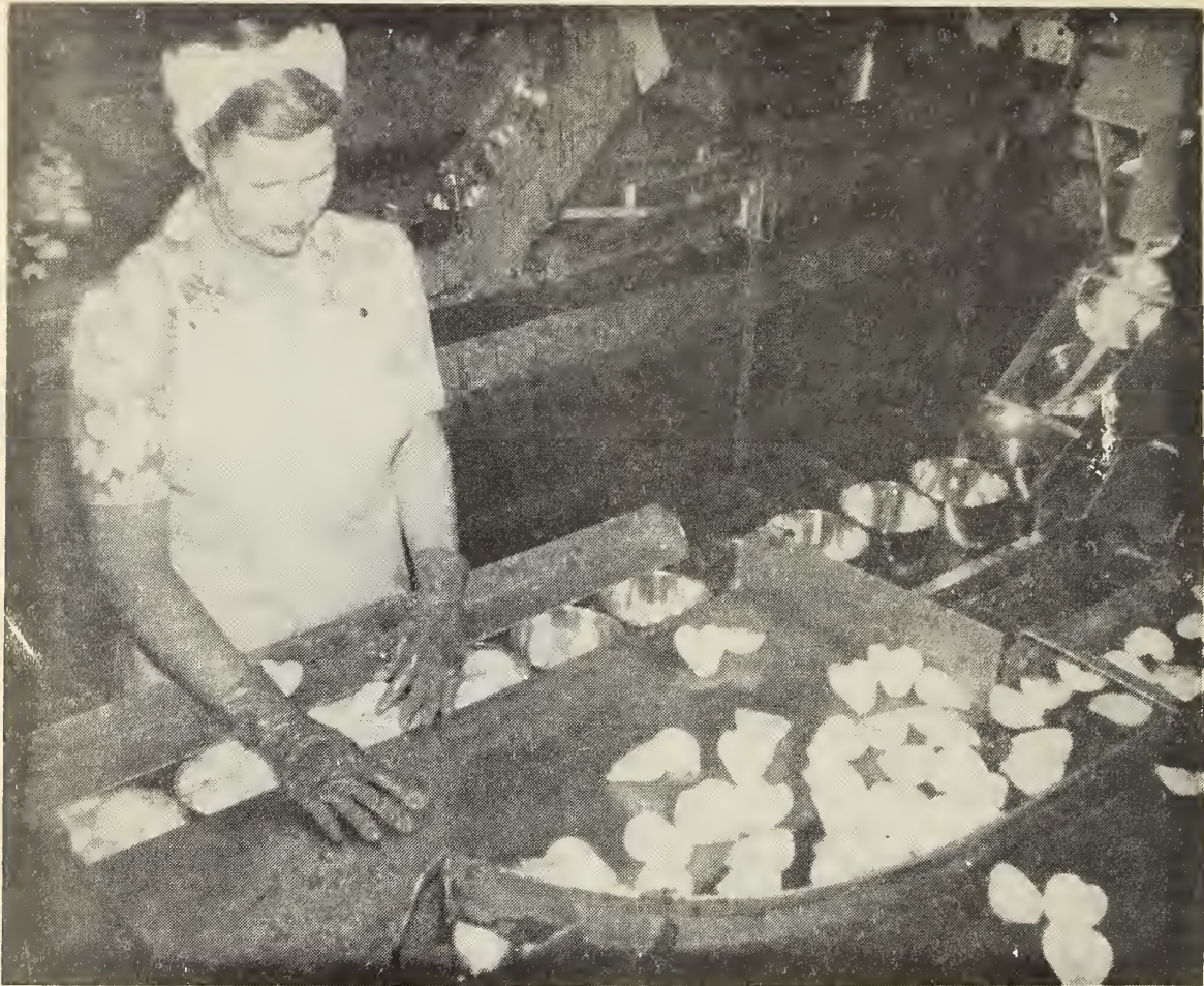
Six No. 10 cans when filled with pears quickly move away and six empty cans take their place automatically before the filler. Tri-Valley Packing Association, San Francisco, Calif.
