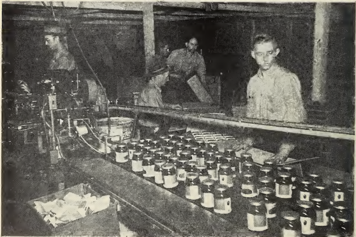
To prevent slipping, adhesive on these newly labelled jars of ripe olives is allowed to "set" before the jars are placed in cases. Lindsay (Calif.) Ripe Olive Co.
