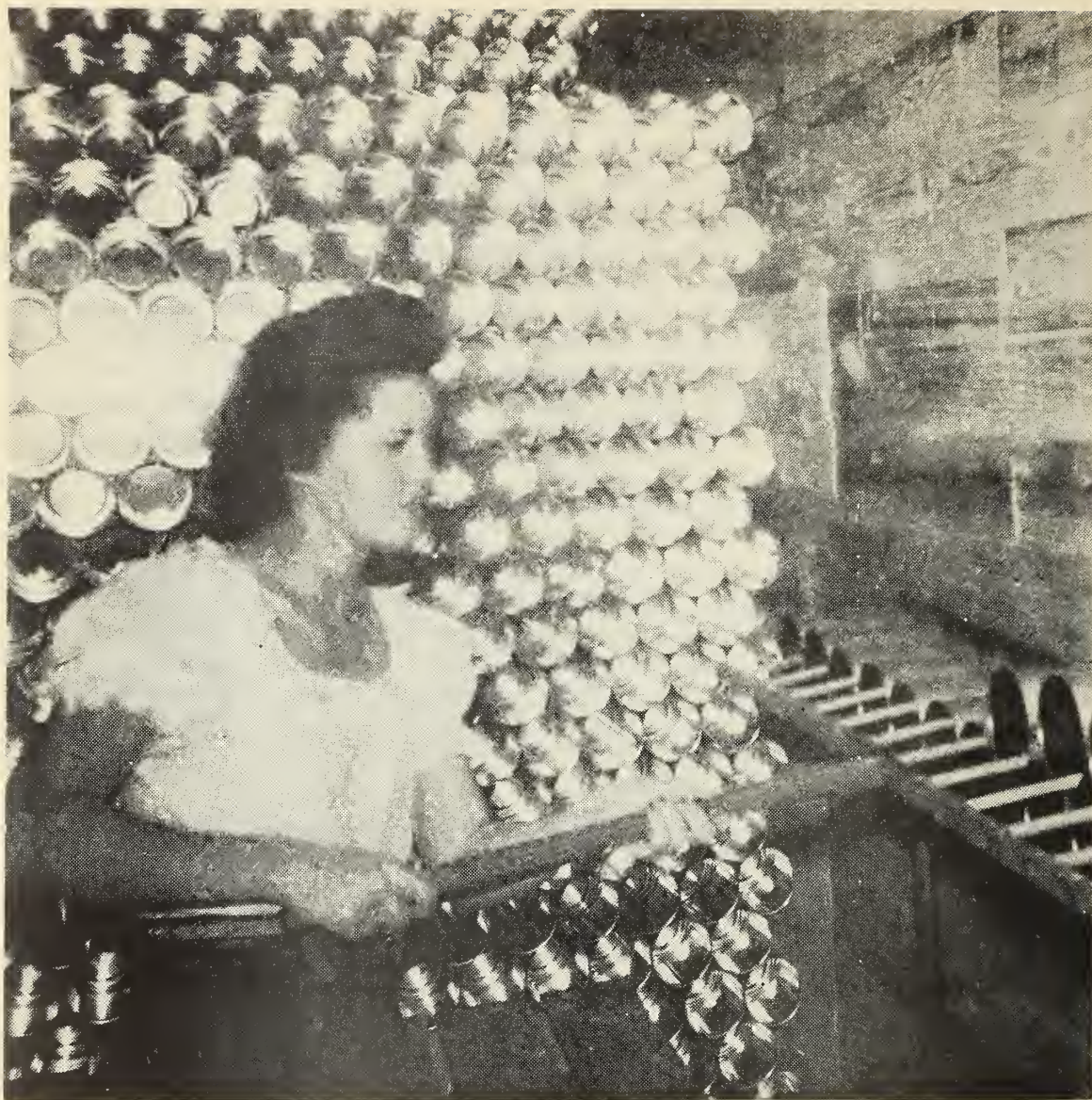
The empty cans are put on the runway with forks, then go through the can washer and directly to the juice filler. Exchange Orange Products Co., Ontario, Calif.
