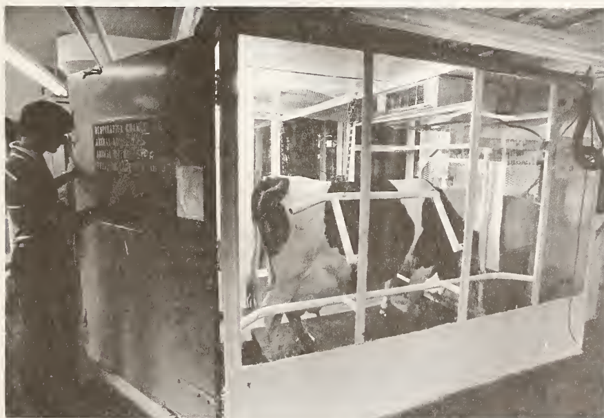
A Holstein cow in a respirator chamber at the Beltsville Agricultural Research Center. This chamber, one of six, is used to determine the energy requirements of dairy cows. The unusual facility was established in the 1960's and continues to operate. Scientist Gordon Haaland records data on cow about to be tested.
