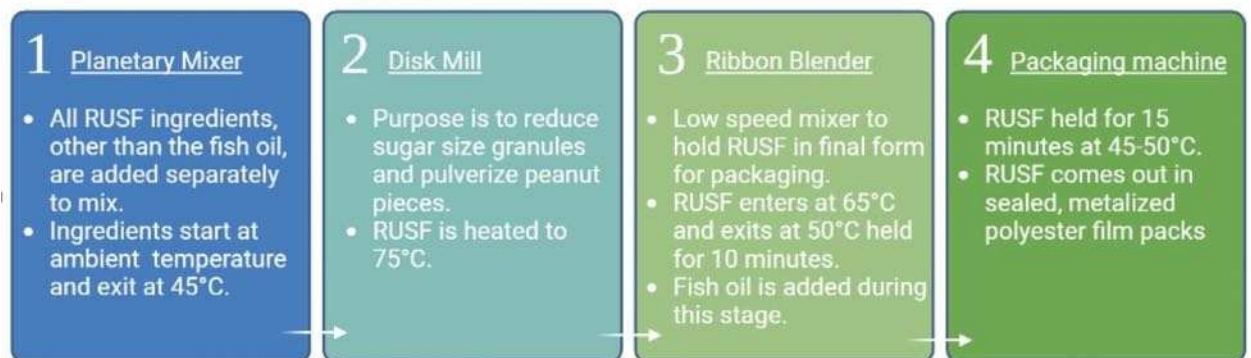
Figure 1: Maternal ready-to-use supplementary food manufacturing process
