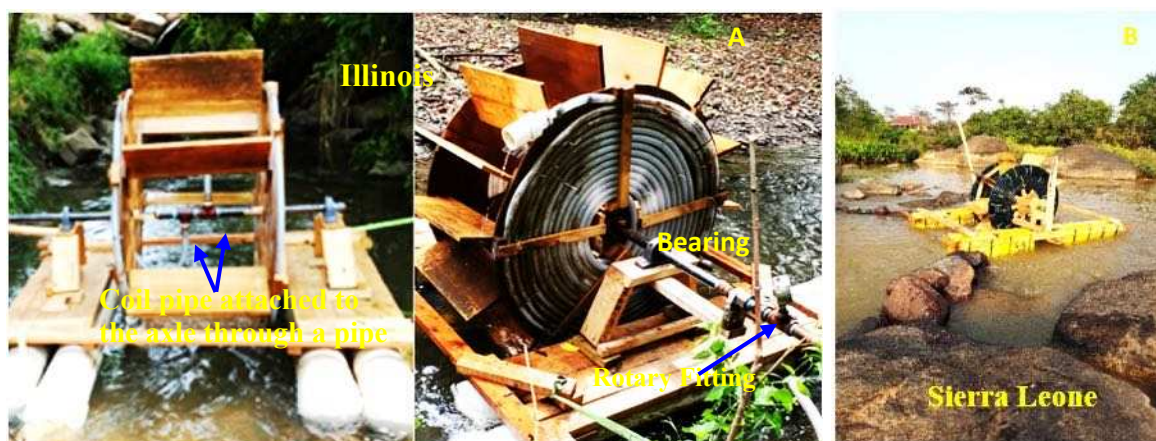
Figure 2: The field-type wheel testing pump (a) in Illinois (with bearings) and (b) in Sierra Leone (without bearings)
