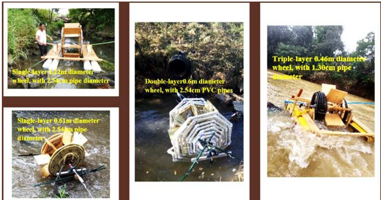
Figure 5: Field setup for data collection on different wheel diameters
