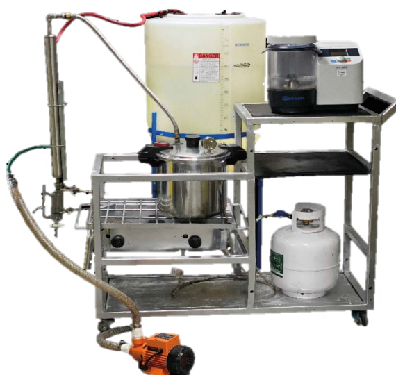
Figure 1. Pilot-scale hydrodistillation apparatus by Armenta et al. , 2023.
