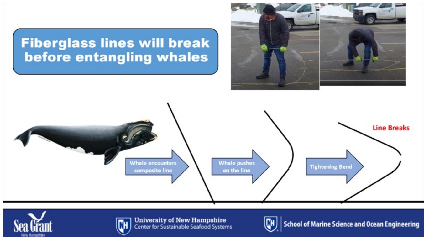
Figure 30. Illustration of a whale encountering a fiberglass rod and bending it until it breaks.
