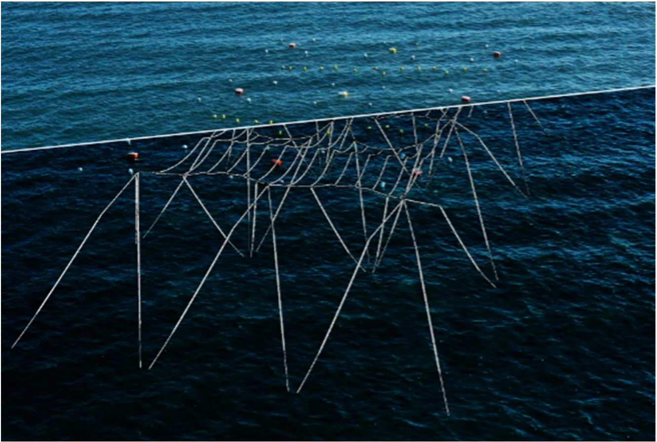
Figure 32. A composite image: a three-dimensional rendering of the mooring and cultivation pilot scale system deployed in Saco Bay, ME with an overlaid photo of the actual surface components at the site.
