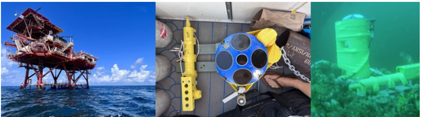
Figure 41. (left) South Pass 83 oil platform, (center) ADCP, CTD, and PAR sensors, (right) sensors in place on South Pass 83.
