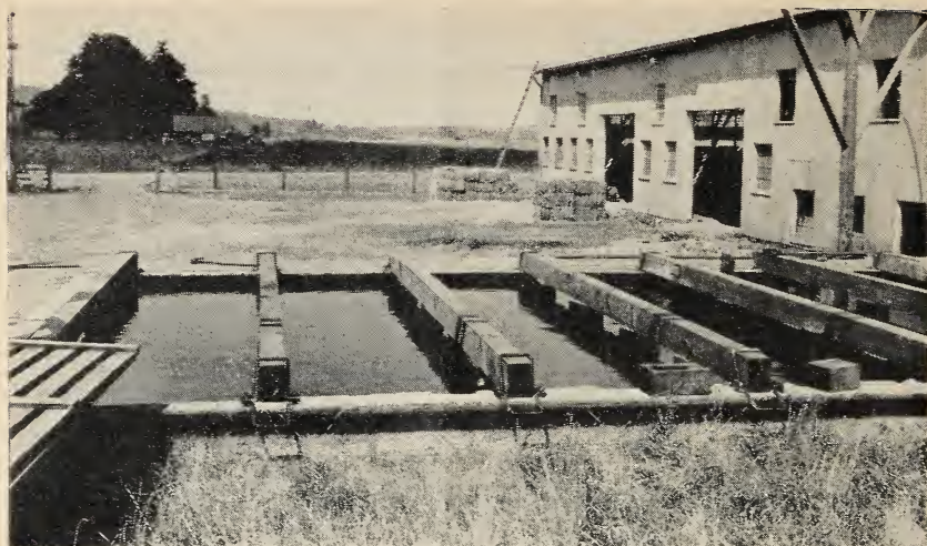
FIGURE 5.—Open tank showing how heavy cross timbers are held in place. Timbers are used over grates for holding the flax straw under water for retting. One of the tanks has been filled with straw, but the grates and timbers have not been placed.
