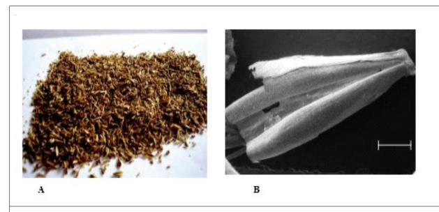
Figure 2: (A) Appearance of Spent Grains and (B) Micrograph of Spent Grains by Scanning Electrons Microscopy with 45 Folds Magnification (Mussatto *et al.*, 2006b)
