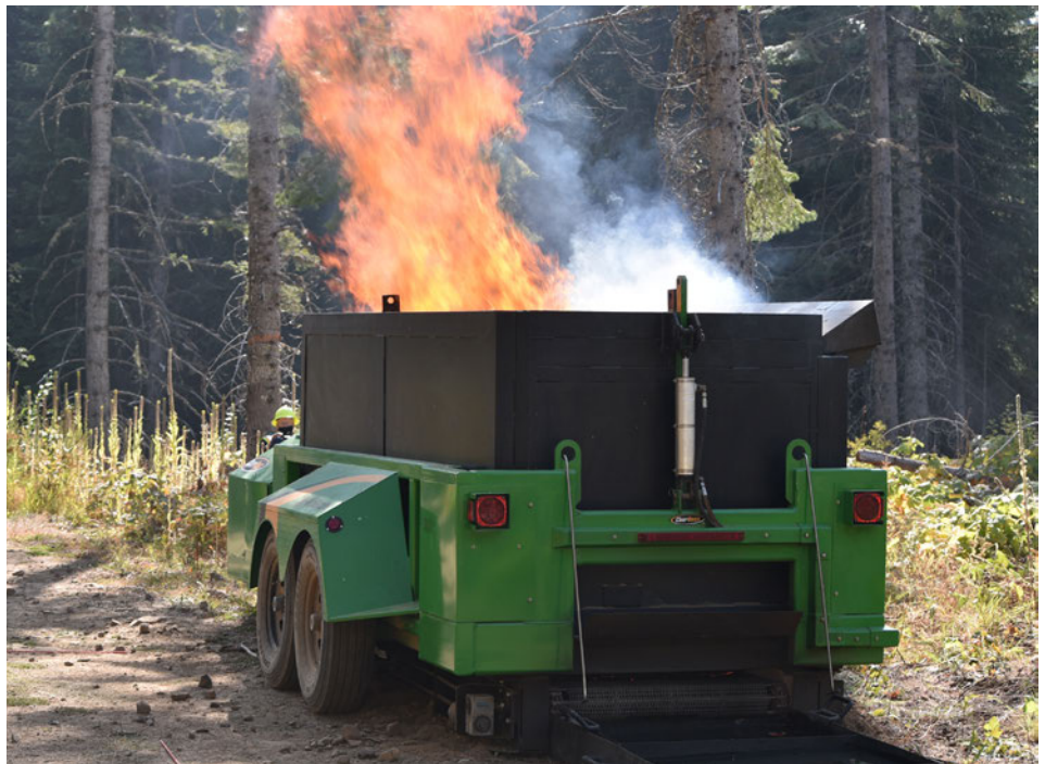
The CharBoss is an air curtain burner-style mobile biochar production machine that can consume material from most burn piles with minimal to no preparation. USDA photo by Darcy Weseman.
