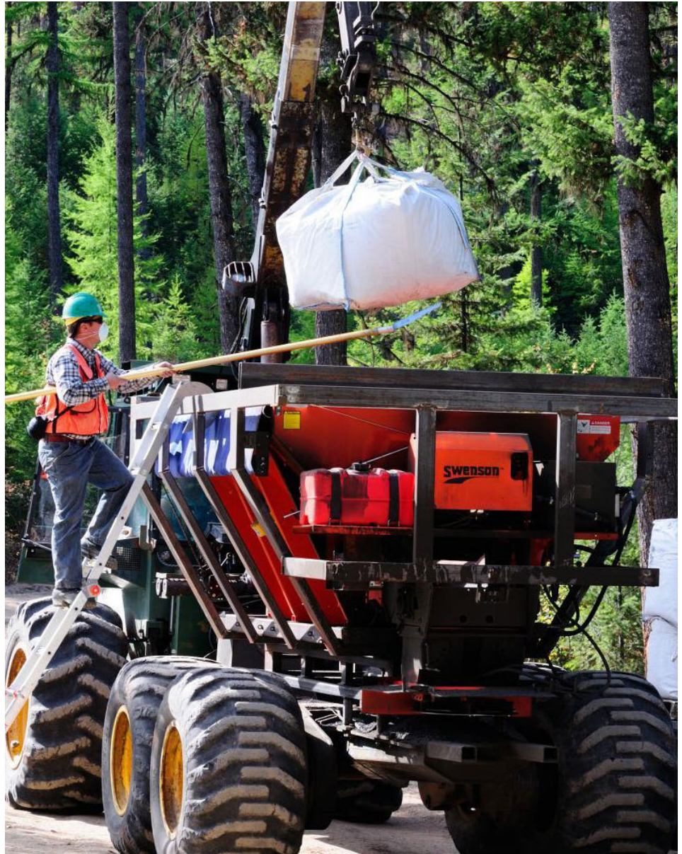
A high-capacity biochar spreader that can be mounted on a log forwarder and used on skid trails and log landings to distribute biochar has been developed by RMRS scientists and the Missoula Technology and Development Center. USDA Forest Service photo.
