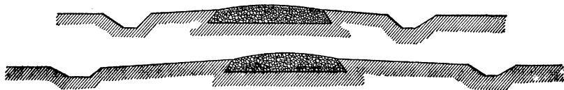
FIG. 131.—Cross sections of Canandaigua roads.
