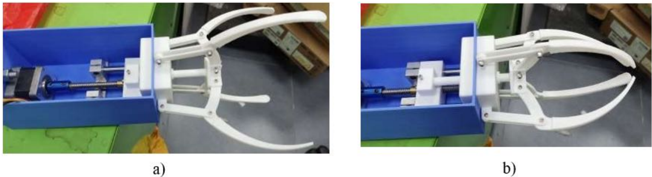
Figure 7: The Gripper in action, a) maximum and b) minimum opening
