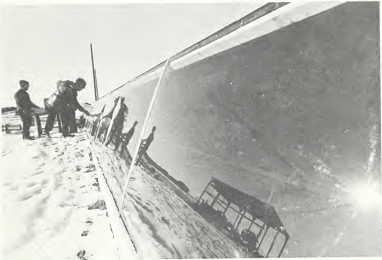
The cover plate of the solar collector being used in this cooperative experiment at Iowa State University, Ames, is a rigid structure made of acrylic plastic. (Courtesy, U.S. Department of Agriculture).
