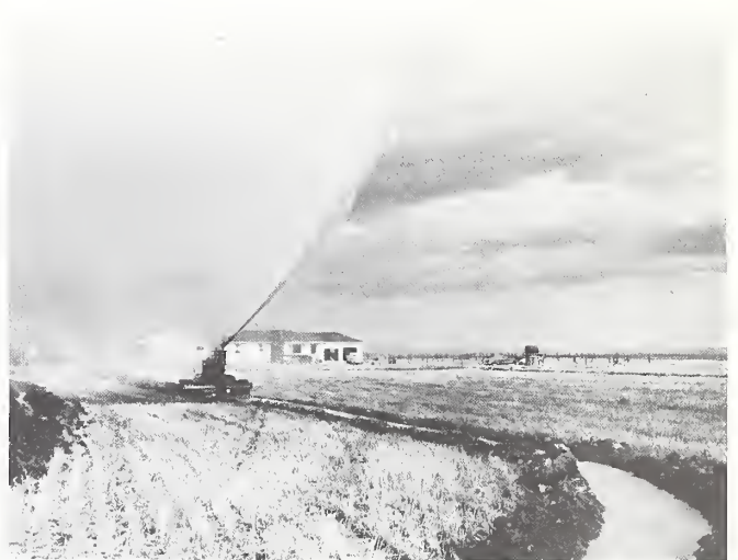
An irrigation machine at work on Blackfeet Indian lands in Montana. The machine draws water from the canal and "rains" over a wide area of surrounding cropland (Courtesy, Bureau of Indian Affairs—Department of the Interior).
