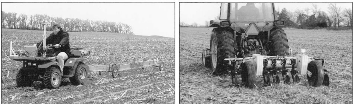
Figure 1 Comparison of the electromagnetic and contact-based EC sensors in the field. (Left) Electromagnetic Geonics EM38 sensor (Right) Veris 3100 contact EC sensor. Source: (Sudduth et al., 2003).
