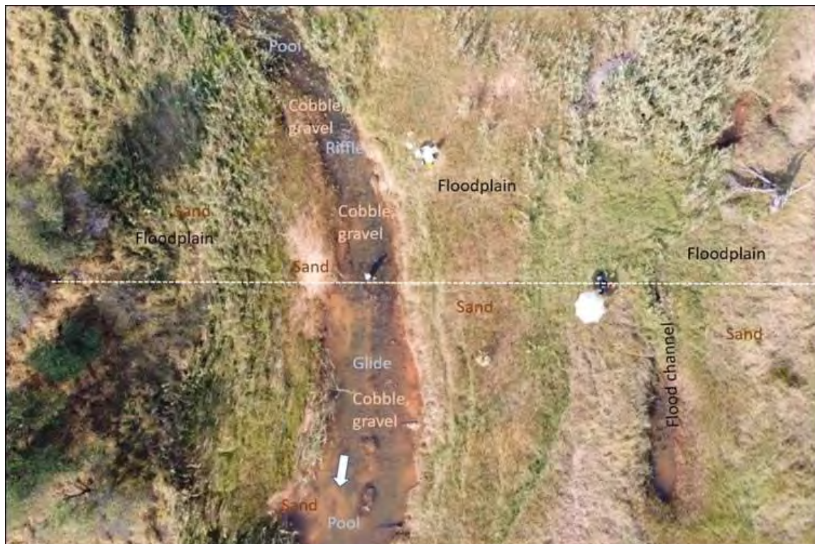
FIGURE 17: ORTHOPHOTO SHOWING MORPHOLOGICAL FEATURES AND SEDIMENT COMPOSITION OF THE MATLABAS RIVER.
