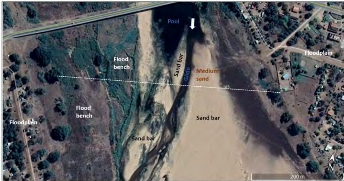
Figure 97). The low-flow channel has a braided pattern that becomes a wandering channel pattern during higher flows (FIGURE 98;
