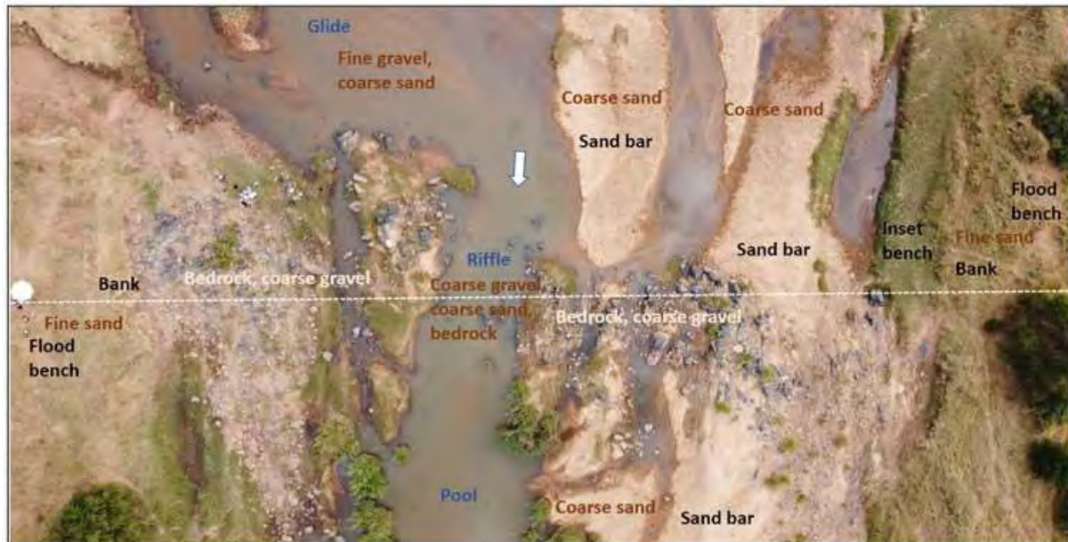
FIGURE 76: ORTHOPHOTO SHOWING MORPHOLOGICAL FEATURES AND SEDIMENT COMPOSITION OF THE GROOT LETABA RIVER.
