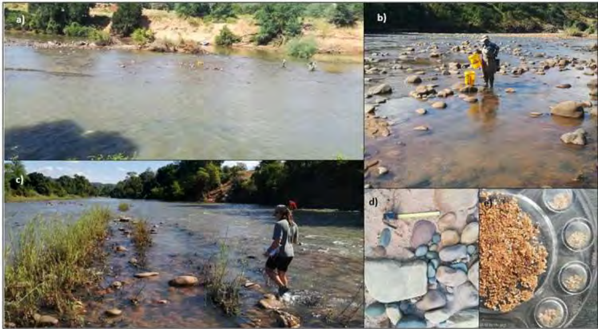
FIGURE 62). The velocity distributions across the riffle and pool are presented in FIGURE 63. Sandy lee bars develop downstream of boulder high points. Small coarse sand and fine gravel deposits are found between the cobble and boulder high points in the slower flow of the riffle. The gravels and cobbles are moderately loose and mobile where not embedded in sand or gravel. Very low embeddedness and imbrication in the flowing water of the riffle. Higher levels of imbrication and embeddedness out of the main flow zone. Bedrock is present along the left bank. The steep right bank is composed of loose medium to coarse sand and show erosion and deposition from the last food. The pools are lined with sand and silt over coble and gravel. Sandy inset benches develop and are covered by reeds.
