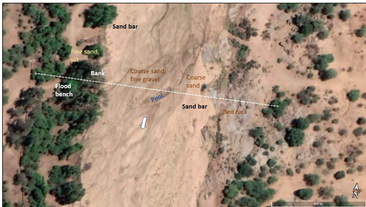
FIGURE 50: ORTHOPHOTO SHOWING MORPHOLOGICAL FEATURES AND SEDIMENT COMPOSITION OF UMZI-Y20C-BEITB (UMZINGWANI RIVER; GOOGLE EARTH IMAGE DECEMBER 2020).
