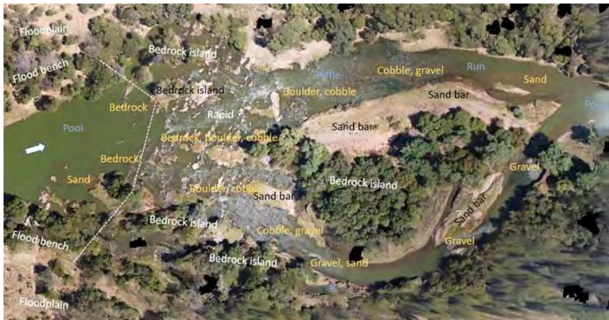
FIGURE 12: ORTHOPHOTO SHOWING MORPHOLOGICAL FEATURES AND SEDIMENT COMPOSITION OF THE LIMPOPO RIVER AT SPANWERK.
