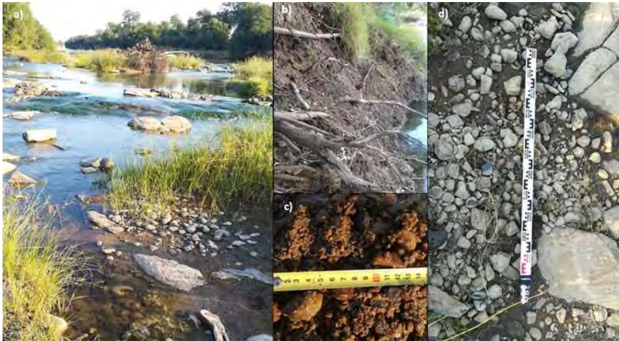
FIGURE 14: SITE IMAGES SHOWING A) EMBEDDED GRAVEL BAR IN THE FOREGROUND AND BEDROCK AND BOULDER SUBSTRATES; B) COHESIVE BANKS SHOWING EROSION; C) FINE GRAVEL AND COARSE SAND DEPOSITED IN THE RIFFLES; AND D) PARTLY EMBEDDED GRAVEL SUBSTRATES
