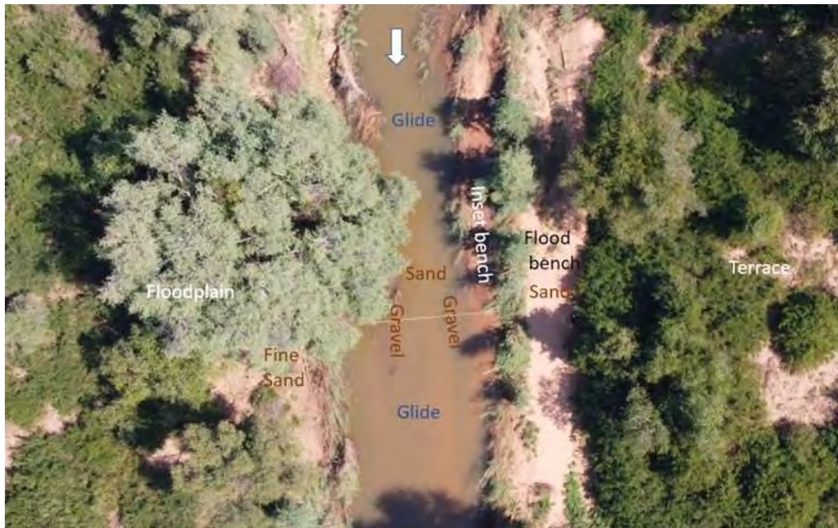
FIGURE 22: ORTHOPHOTO SHOWING MORPHOLOGICAL FEATURES AND SEDIMENT COMPOSITION OF THE LEPHALALA RIVER.
