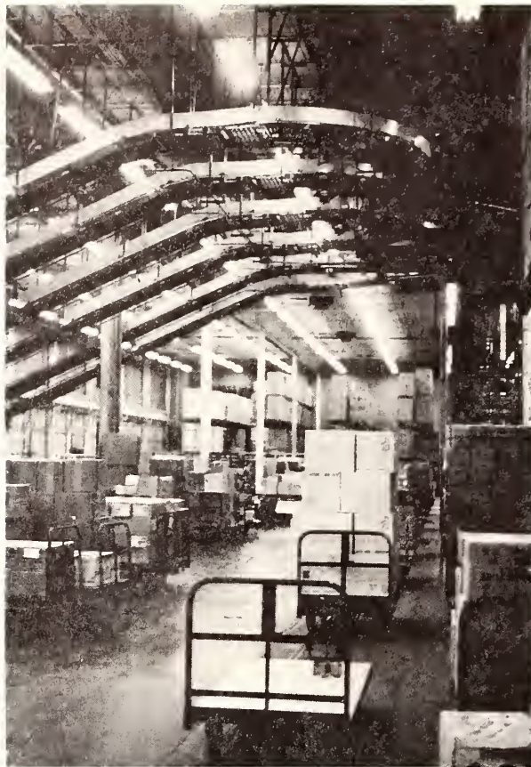
Figure 4.—Declining conveyors leading to shipping doors.
