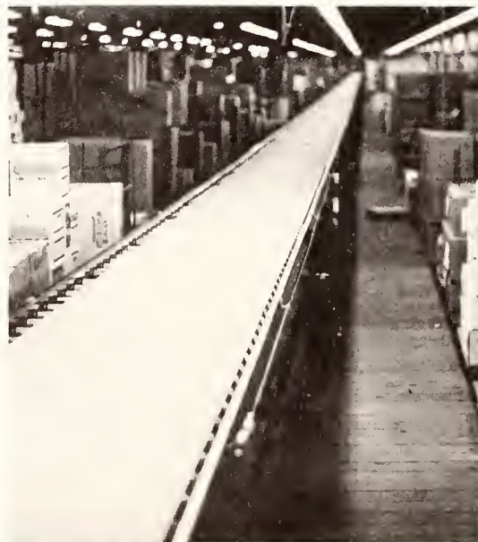
Figure 1.—Conveyor line used for order selecting.
