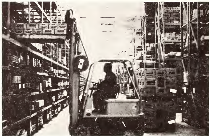
Figure 23.—Forklift truck positioning pallet of products on platform of mechanized selection machine.
