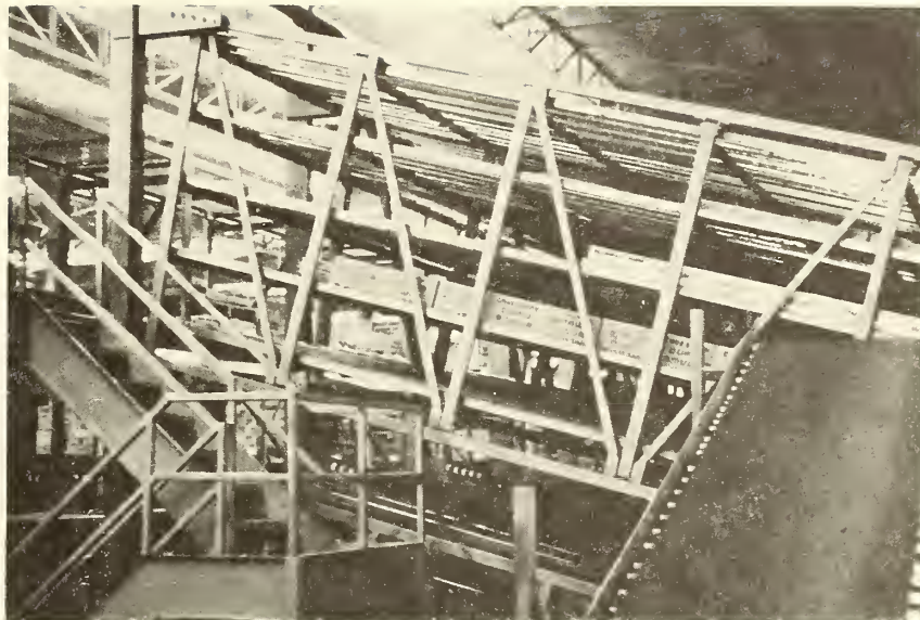
Figure 24.—Upper five levels of inclined chutes on selection machine.
