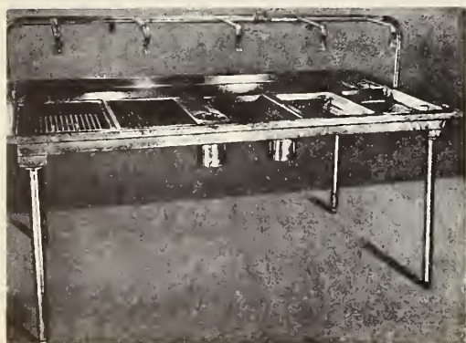
Figure 18. - Metal eviscerating table with individual trays and adjustable sprays.
