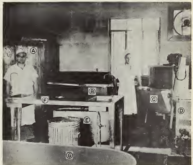
Figure 7. - Plant arrangement and equipment used in one commercial plant: (a) killing and bleeding cabinet, (b) scalding tank, (c) picker, (d) plumping tank, (e) rinsing tank, (f) drawing table, (g) cooling tank.
