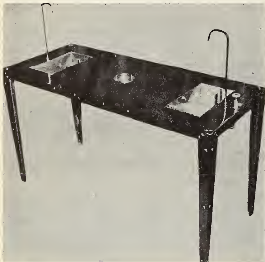
Figure 16. - Metal eviscerating table with sinks and rinsing faucets
