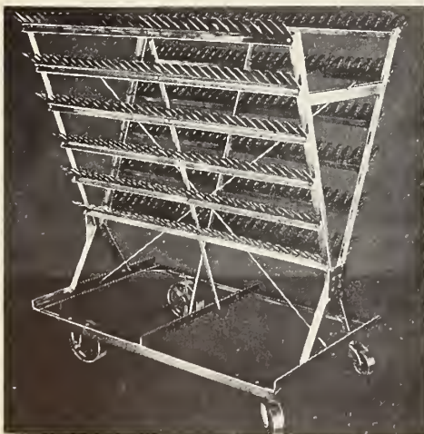
Figure 14. - This movable rack for dry-cooling or draining has a capacity for 180 birds.
