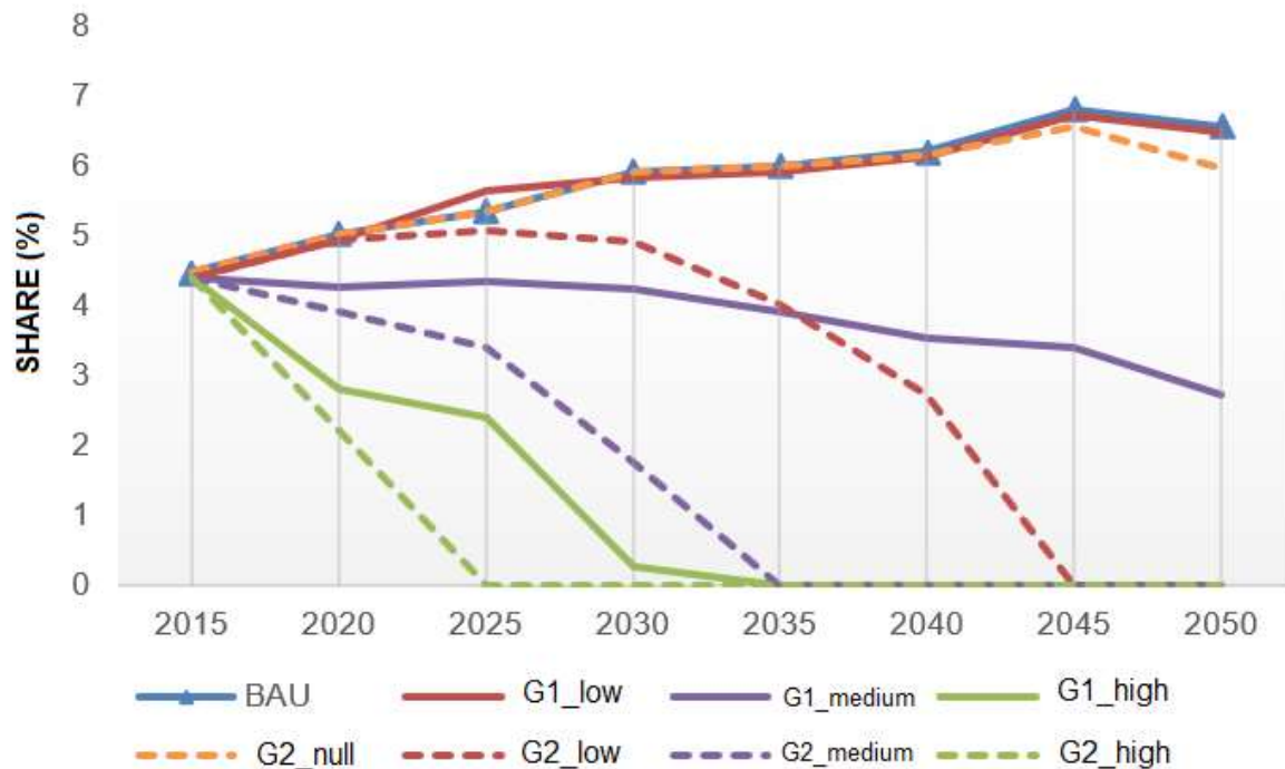
Figure 9 – Share (%) of sugarcane biomass electricity in the generation of energy in the period from 2015 to 2050 for the scenarios simulated in this study (reference scenario, scenarios of group 1 and scenarios of group 2).
