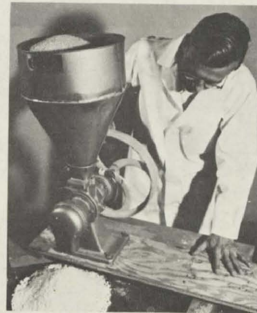
FIGURE 4.—Processing whole soybeans: A, cooking; B, air-drying; C, cracking cooked, dried beans; D, winnowing to separate hulls; E, diagram of winnower operation; and F, hand-grinding meats to flour.
