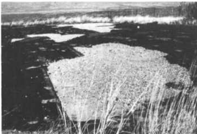
Figure 43.—Catchment treatment destroyed by wind because of the lack of preventive maintenance.
