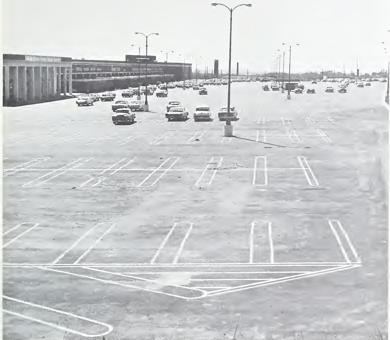
Figure 55.—Extensive buildings, parking lots, and paved streets waterproof most of the land surface in urban and built-up areas, greatly increasing runoff of rainfall.
