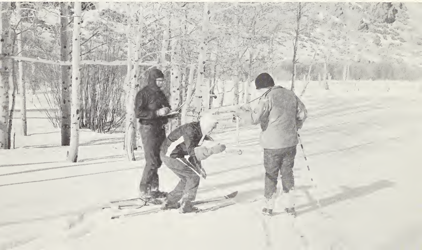
Photograph 17. - Forest Service and Soil Conservation Service snow surveyors weighing a snow sample on an Independence Mountains snow course, Humboldt National Forest. North Fork Sub-Basin.
