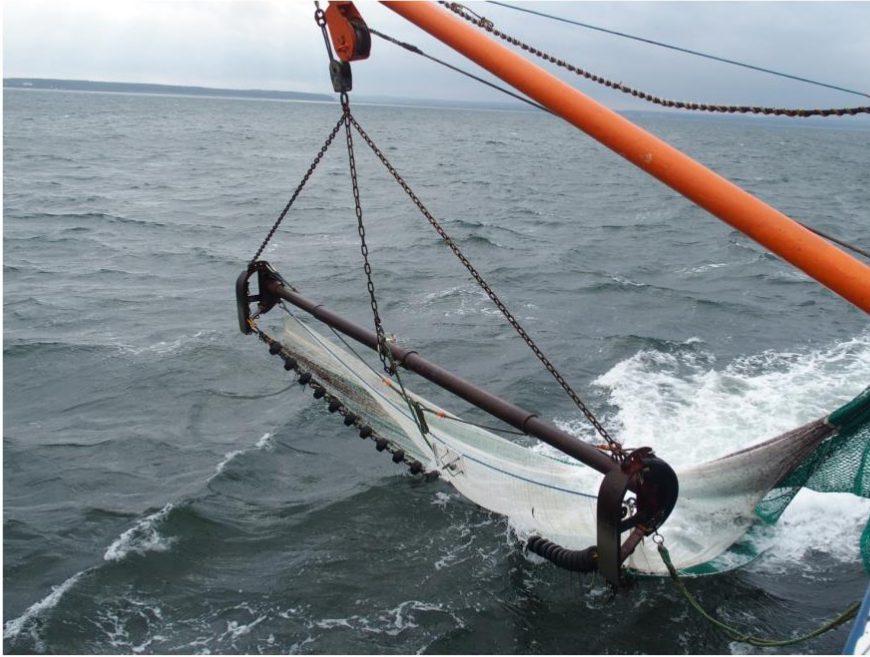
Abbildung 26: Schlepp-Hahnepot am Kurrbaum Figure 26: towing bridles on the trawl beam
