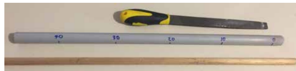
Figure 10.4. Sharpened 20mm pipe and 13mm dowel (Source: Richard Stirzaker)
