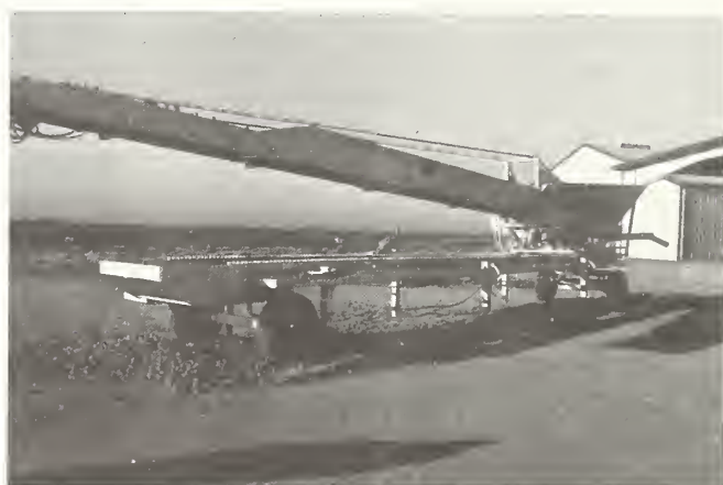
Figure 22. A Special Conveyor to Bulk Load Containers for Export.
