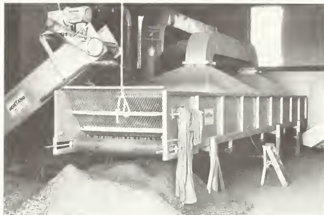
Figure 18. A Small Cube Cooling Apparatus.
