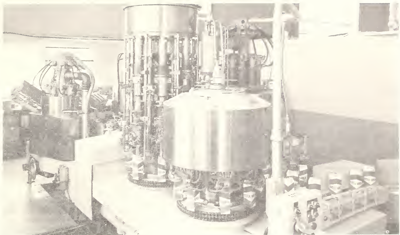
At a speed of two per second, this machine forms cartons, fills them, and seals them. Various sized containers can be made with a simple changeover.
