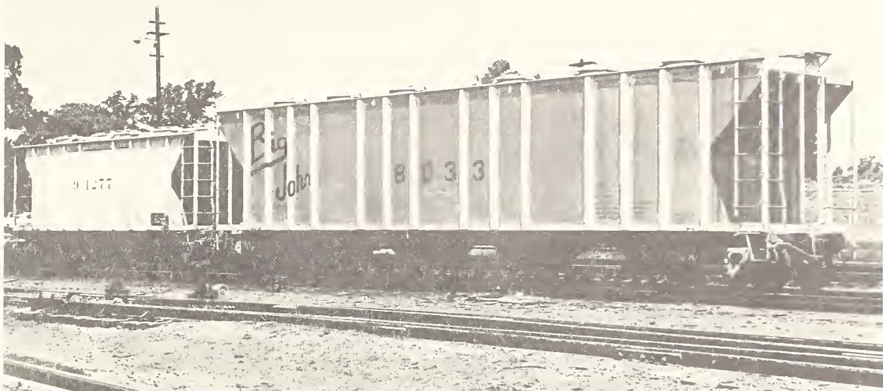
Big John and its little brother. The 100-ton plus capacity Big John is made of aluminum and has 12 roof hatches and 8 discharge hoppers for fast loading and unloading. Little brother is a standard size steel covered hopper car. (Photo courtesy of Southern Railway.)
