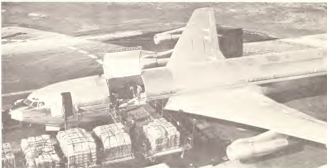
Mechanized loading device, with push-button control, unloads and reloads a 90,000-pound capacity jet freighter in 40 minutes. (Photo courtesy of American Airlines.)
