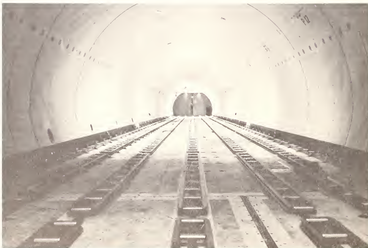
The interior of this jet-freighter is equipped with rollers, permitting easy movement of palletized cargo. The freighter is 102 feet long and can carry 45 tons of cargo. (Photo courtesy of American Airlines.)
