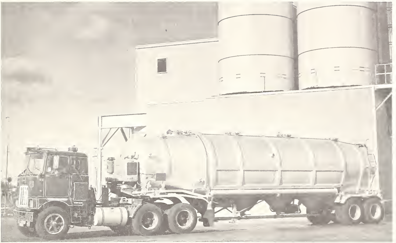
Hopper trailer with pneumatic unloader used for hauling flour and feed. (Photo courtesy of Butler Manufacturing Co.)
